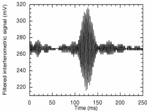
**Fig. 5.** Coherent addition of the signals injected by the two telescopes into the single mode coupler: a typical single-scan interferogram obtained on  $\alpha Her$ , filtered at the optical bandpass. Resolution is limited on the temporal axis by the finite sampling rate (2092 Hz), and in the detected signals by the dynamic of the data acquisition board (2.4 mV of resolution).
