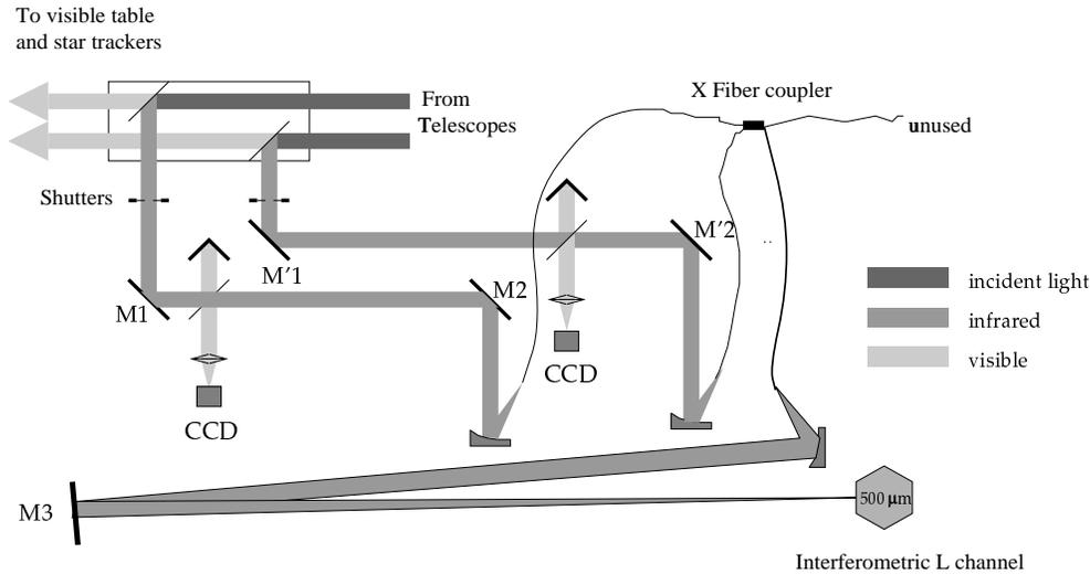
**Fig. 1.** Optical lay out of the TISIS combination table in the L band. A single X coupler is used for coherent combination of the beams coming from the 2 telescopes. There is only one interferometric output and no monitor of the signals coupled into the fibers.
